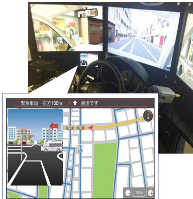
Fig. 4-3 Forward screen and car-navigation display
