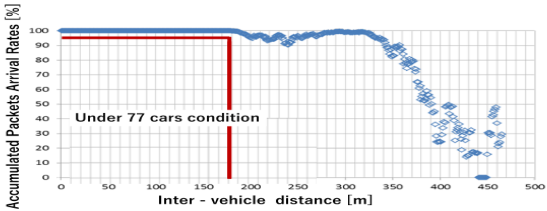
Fig. 3-12 Packet arrival rate in communication between car and car
