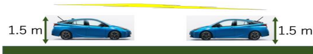
Fig. 3-11 Antenna height in communication between car and car
